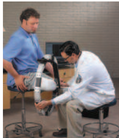
Omega Tracer T-Ring™ II captures residual limb shape in moments.
