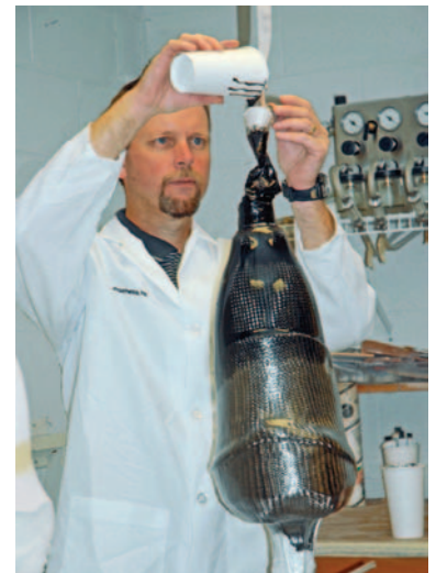
Adding catalyst-pigment mixture to activate socket lamination.
